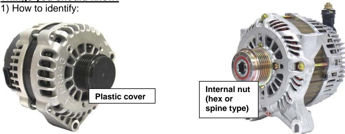
2) Alternator Spin Test. Many customers like to hand spin the alternator from the pulley... just to make sure it turns smoothly. If it has a pulley clutch it will only spin one direction (the clutch will free-spin the other way).
