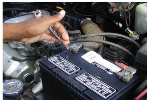
**3 Remove the start terminal lead (small lead).**
