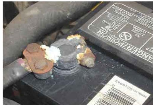
Corroded/Loose connections. Spliced on cable terminals are a **common** source of problems. Replace bad cables and clean all corrosion from terminal ends and cables.
