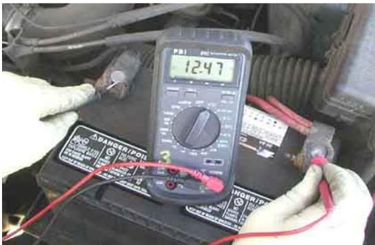
1) Check to make sure the battery is charged to 12.4-12.6 volts. **If it is not**, check the battery fluid level (if it is low, add distilled water to bring the level up to the fill line) and **charge the battery now**. 2) Now turn on the headlights if the voltage drops below 12.1v, the battery may be bad.
